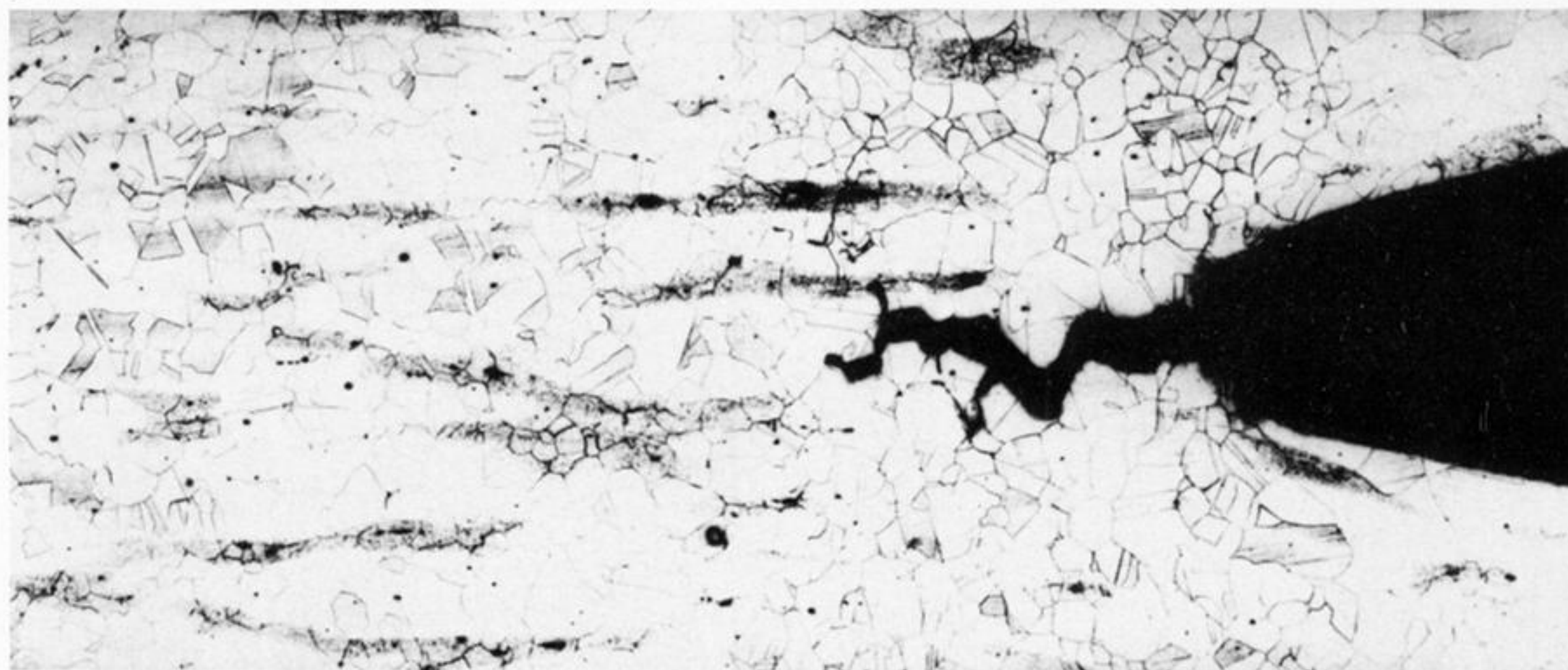
FIGURE 16. Comparison of (a) computed failure path, \omega \geq 0.999 , with (b) mid-thickness micrograph taken from the minimum section of an externally cracked specimen in 316 stainless steel at t/t_1 = 0.6 .
